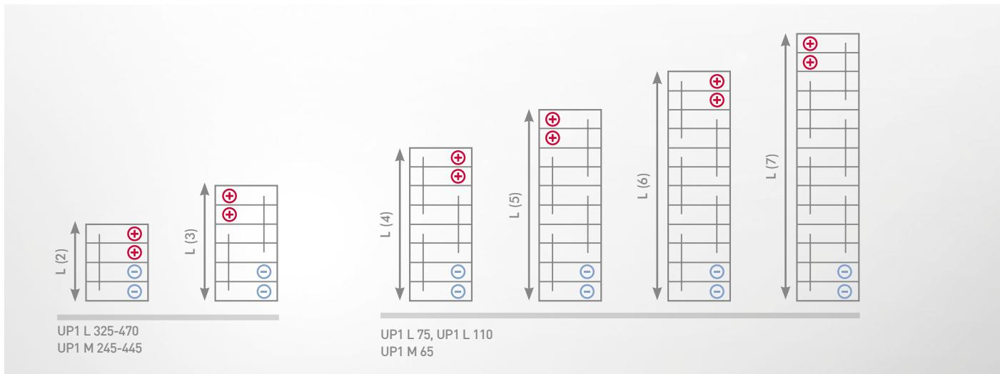
With 2-6 bolts per pole, crosswise mounted on racks
