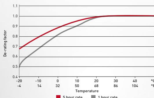
Temperature de-rating factors for M type cell
